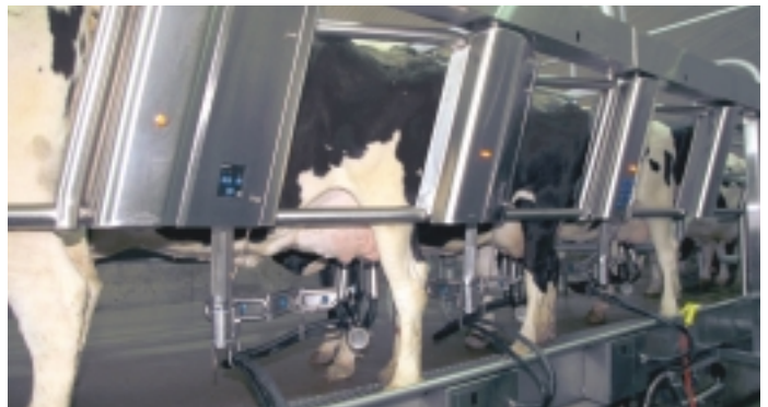
The indexing system allows for gentle and correct positioning of cows every time.
